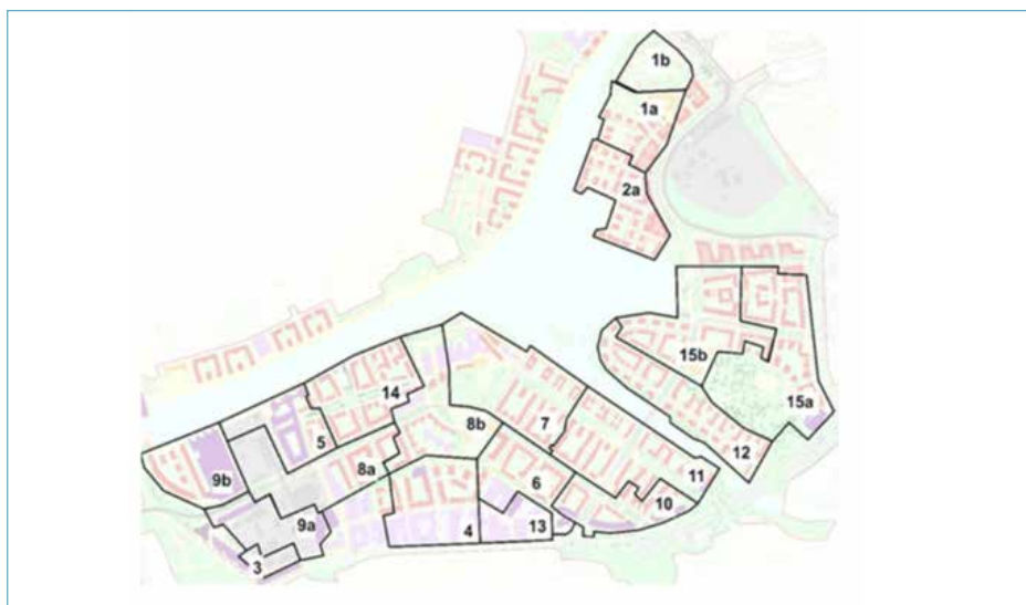
figure 6: the areas serviced by each of the substations in Hammarby Sjöstad (Monika Topel)
