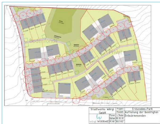
figure 13: (schematic) distribution of the geothermal heat probes over the project site (Stadtwerke Wörgl GmbH)
